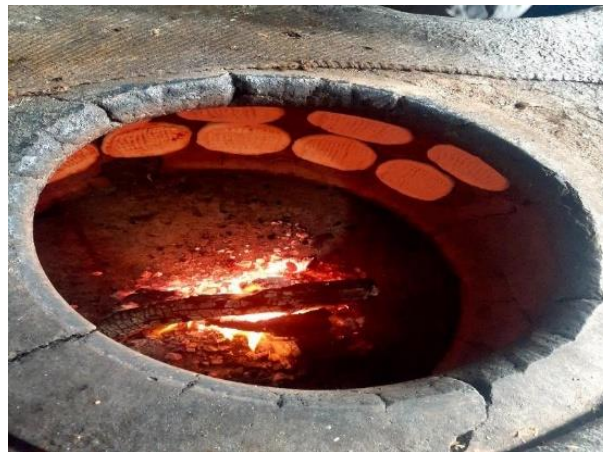
Fig. 1: Old Design of the Tandoor Under Operating Conditions.
