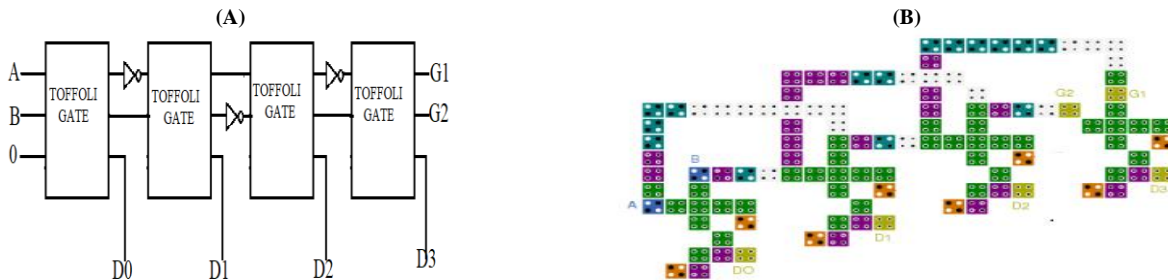
Fig. 3: (A) Proposed 2:4 Decoder Logic Diagram (B) QCA Layout.
