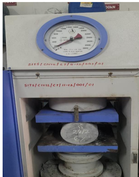
Fig. 11: Split Tensile Strength Test on Compression Testing Machine
