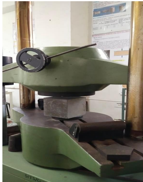
Fig. 10: Compression Strength Test on Universal Testing Machine
