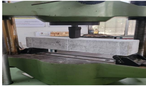
Fig. 12: Flexural Strength Test on Universal Testing Machine
