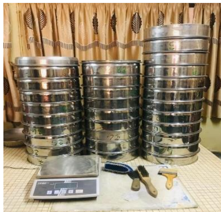
Fig. 3 : Shows Images of the Sieves, Scales and Brushes Used.
