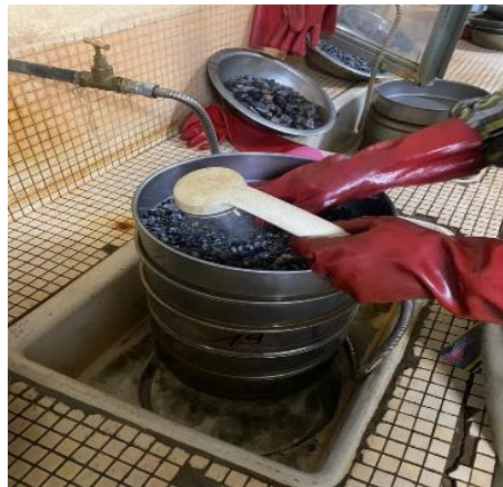
Fig. 2: Photo of Sieve Washing.
