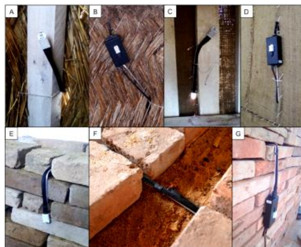
Fig. 9: ECCs equipped with data logger [30].
