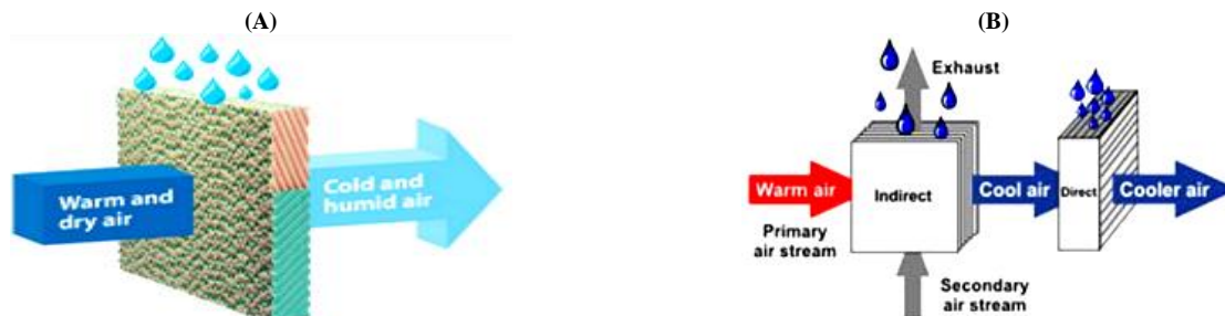
Fig. 2: Evaporative Cooling. (A): Direct, (B): Indirect.
