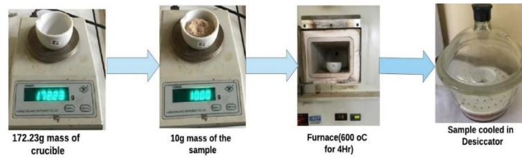
Fig. 6: Experimental Procedure of AC (%) Estimation.
