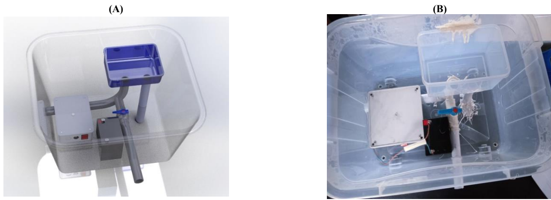
Fig. 2: (A) CAD Model of the Pipeline Leakage Monitoring System (B) Pictorial View of the Physical Model.
