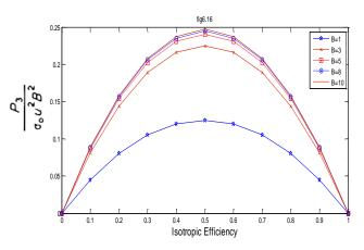
Figure 8 Isotropic Efficiency for Hall generator
