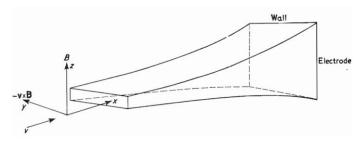
Figure 1: Basic MHD duct
