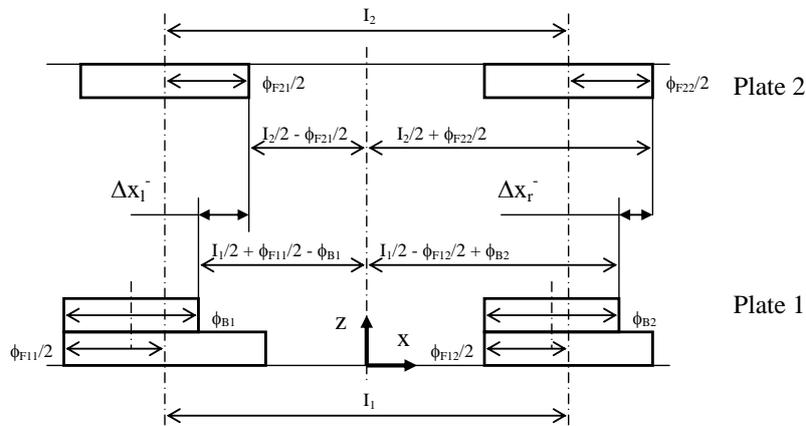
Fig. 8: Displacement of the Second Plate as Regards to the First Plate along the Negative X-Axis.
