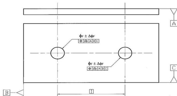
Fig. 1: Part with Two Holes.
