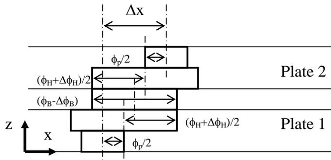
Fig. 3: Maximum Deviation between the Top Surface of the Second Plate and the Bottom Surface of the First Plate along the X-Axis.
