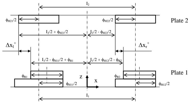
Fig. 7: Displacement of the Second Plate as Regards to the First Plate along the Positive X-Axis.
