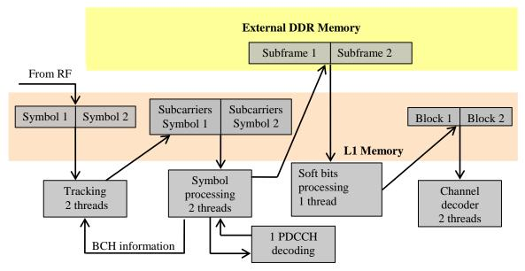
Fig. 5: LTE Partitioning on SB3500
