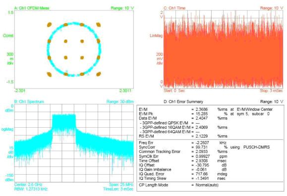
Fig. 7: Snapshot From Agilent MXK N9026A Signal Analyzer
