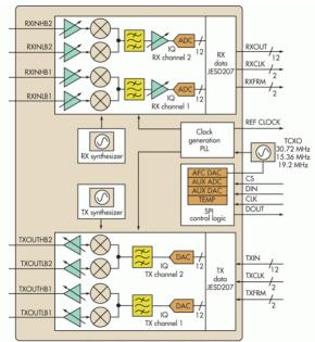
Fig. 2: Maxim Multistandard 3G/4G Transceiver [2].
