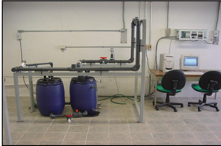
Fig. 1: A) Loop Reactor System Designed and Built for Corrosion Testing.
