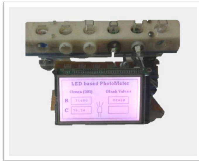
Fig. 10: The LED Based Spectrophotometer Device.
