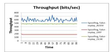
Fig. 9: Throughput of (AODV, GRP and OLSR) with DOS Attack for 16 Nodes.
