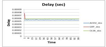
Fig. 5: Packet End-To-End Delay of AODV, GRP and OLSR with Attack for 16 Nodes.
