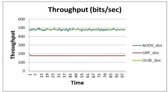
Fig. 2: Throughput of (AODV, GRP and OLSR) with Dos Attack for 16 Nodes.
