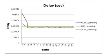
Fig. 7: Packet End-To-End Delay of AODV, GRP and OLSR with Attack for 16 Nodes.
