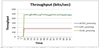
Fig. 6: Throughput of (AODV, GRP and OLSR) with DOS Attack for 16 Nodes.
