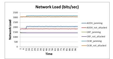
Fig. 8: Network Load of (AODV, GRP and OLSR) with and without Attack for 16 Nodes.
