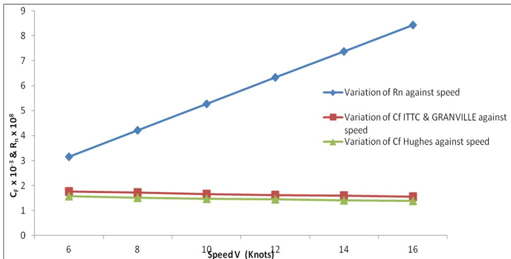
**Fig. 1:** Total Frictional Resistance Coefficient and Reynolds Number against Speed for Cargo Ship.
