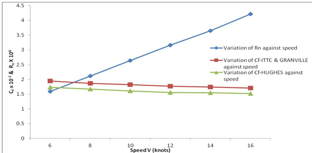
Fig 2: Total Frictional Resistance Coefficient and Reynolds Number against Speed for Ocean-Going Tug.
