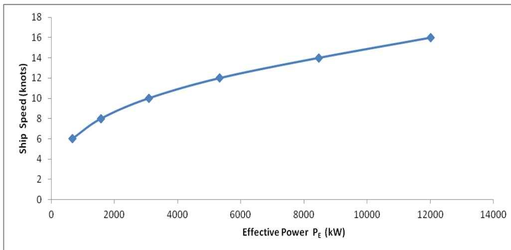
Fig. 3: The Ship Speed of the Containership against the Effective Power Developed.
