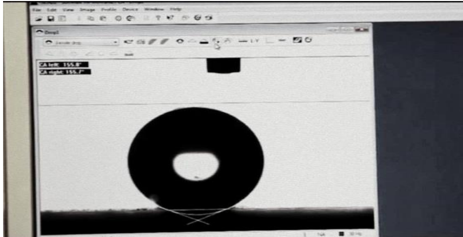
Fig. 6a: Water Drop Image on Insulator Tiny Sample (S 1 ).
