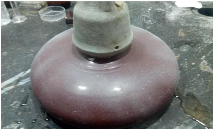
Fig. 12 (B): Coated Insulator without Any Dust Particle.
