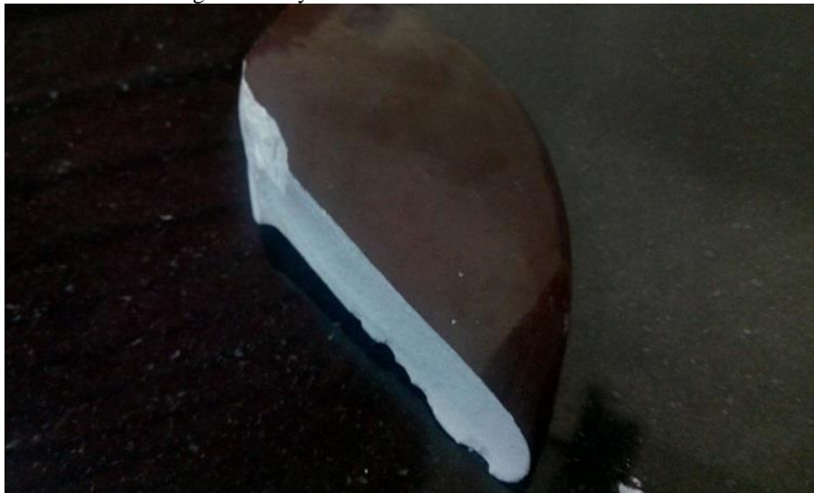
Fig. 14 (A): Broken Porcelain Insulator During Rain Test.
