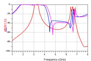
Fig. 3: Transmission Coefficient of Filter versus Frequency of Bandpass with Defected Ground Plane for Different Radii of Metallic Patches.
