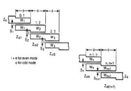
Fig. 1: Parallel-Coupled Transmission Line Resonator filter
