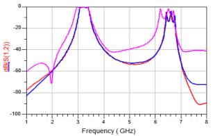
Fig. 4: Transmission Coefficient of Filter versus Frequency of Bandpass with Defected Ground Plane for Different Radii of Slots.
