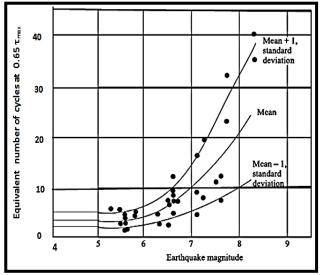
Fig. 7: Equivalent Numbers of Uniform Stress Cycles Based on Strong Component of Ground Motion (Modified from Seed Et Al., [19]).
