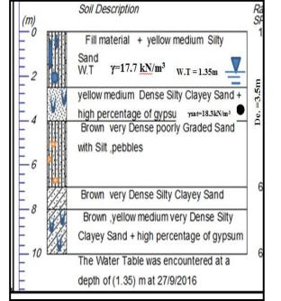
Fig. 5: Soil Profile for Site K3 in Kerbala City and Some Physical Properties.
