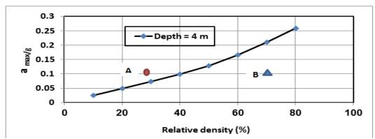
Fig. 11: Plot of  $A_{max}/G$  versus Relative Density for Prediction of Liquefaction Potential in Site K3 in Kerbala City, N = 3.5,  $D_{50} = 0.2$  Mm.
