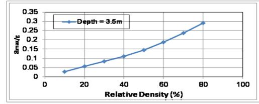
Fig. 12: Plot of Amax/G versus Relative Density for Prediction of Liquefaction Potential in Site N.K.L in Kerbala City, N = 3.5, D<sub>50</sub>= 0.15 Mm.
