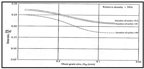
Fig. 10: Stress Ratio Causing Liquefaction of Sands in 3.5, 10 and 30 Cycles (Modified from Seed and Idriss, [5]).
