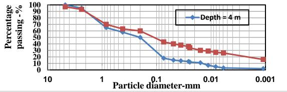
Fig. 3: Grain Size Distribution Curves to Site (K3) in Kerbala City.
