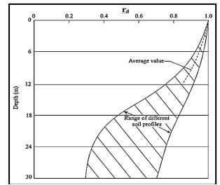
**Fig. 8:** Reduction Factor to Estimate the Variation of CSR with Depth below the Ground Level or Gently Sloping Ground Surface (after Seed and Idriss, [5]).
