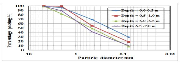
Fig. 4: Grain Size Distribution Curves for Site (N.K.L) in Kerbala City.
