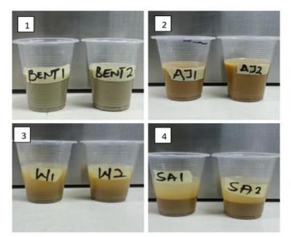
Fig. 2: Prepared Samples; 1). Bentonite Mud. 2) Mud Prepared from Clay Samples from Ajumako. 3) Mud Prepared from Clay Samples From Winneba & 4) Mud Prepared from Clay Samples from Saltpond.
