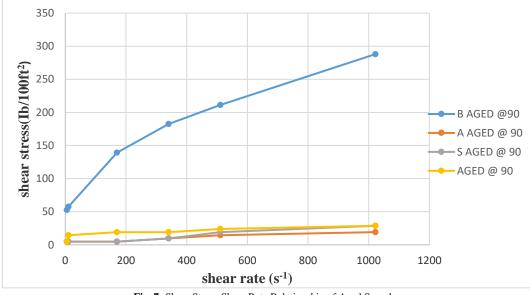
Fig. 7: Shear Stress-Shear Rate Relationship of Aged Samples.
