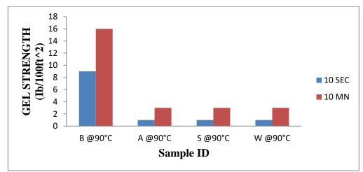
**Fig. 4:** Gel Strength against Samples at Aged for 8hours at 90<sup>o</sup>C.
