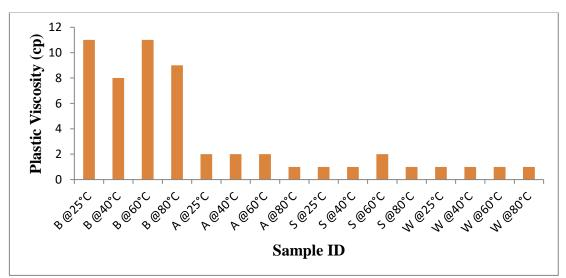
Fig. 5: Plastic Viscosities of Unaged Samples.
