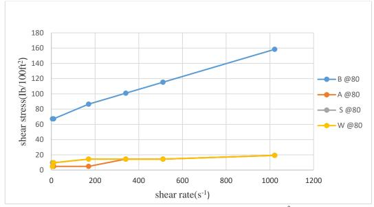
Fig. 8: Shear Stress-Shear Rate Relationship of Unaged Samples at 80°C.
