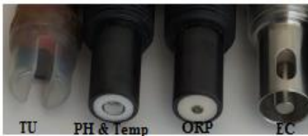
Fig. 5: Sensors deployed in pipeline
