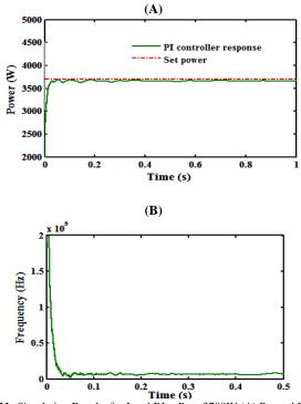
Fig. 11: Simulation Results for Load RL<sub>1</sub>,  $P_{set}$ = 3700W (A)  $P_{set}$  and  $P_0$  with PI Controller (B)  $F_{sw}$  Time Evaluations.
