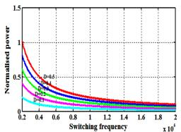
**Fig. 3**: Normalized Power Graph as the Function of the  $F_{sw}$  with Respect to the Various Operating Points.
