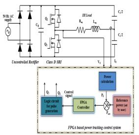
Fig. 1: Schematic of the Class D Resonant Inverter Based IC System.
