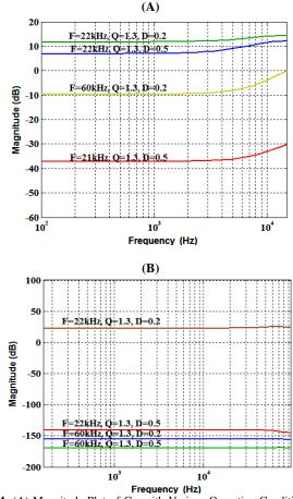
**Fig. 4:** (A) Magnitude Plot of  $G_{pd}$  with Various Operating Condition (B) Magnitude Plot of  $G_{pf}$  with Various Operating Condition.
