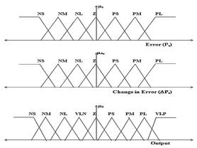
Fig. 8: Membership Functions of Input and Output Variables.
