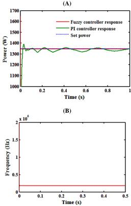
Fig. 14: Simulation Results for Load RL<sub>2</sub>,  $P_{set}$ = 1350W (A)  $P_{set}$  and  $P_0$  with Various Controllers (B)  $F_{sw}$  Time Evaluations with FLC.
