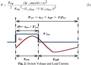
Fig. 2. Switch Voltage and Load Current.
