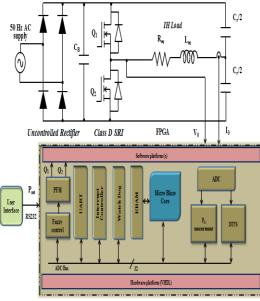
Fig 15: FPGA Implementation of the Proposed Fuzzy Logic Controller.
