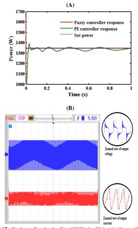
**Fig 17:** Hardware Results for  $P_{set}$ =1350W for RL1: (A) Output Power Waveform Output Waveforms with PI and FLC Calculation (B)  $V_0$  (Blue) 100 V/Div and I<sub>0</sub> (Red) 8 A/Div, 10 Ms/Div, at the Target Set-Point.
