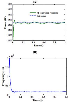
Fig. 13: Simulation Results for Load RL<sub>2</sub>,  $P_{set}$ = 1350W (A)  $P_{set}$  and  $P_0$  with PI Controller (B)  $F_{sw}$  Time Evaluations.
