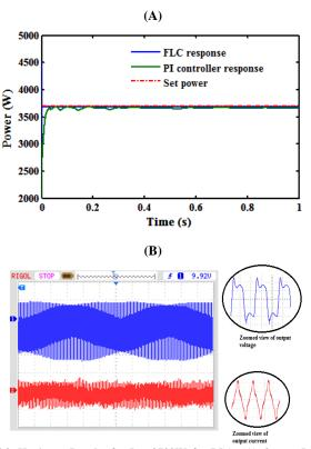
Fig 16: Hardware Results for  $P_{set}$ =3700W for RL1: (A) Output Power Waveform Output Waveforms with PI and FLC Calculation (B)  $V_0$  (Blue) 200 V/Div and  $I_0$  (Red) 15 A/Div, 10 Ms/Div, at the Target Set-Point.
