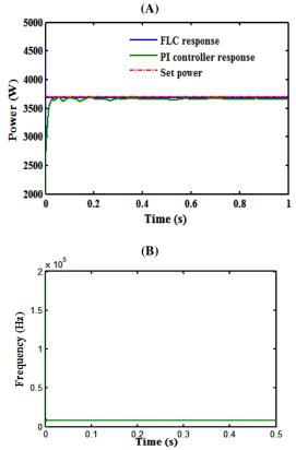
Fig. 12: Simulation Results for Load RL1,  $P_{set}$ = 3700W (A)  $P_{set}$  and Powith Various Controllers (B)  $F_{sw}$  Time Evaluations with FLC.
