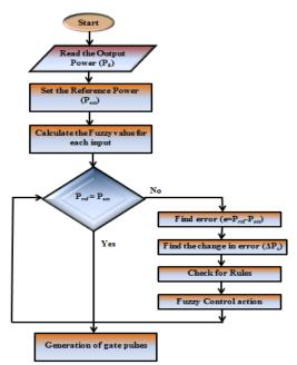
Fig. 10: Flow Chart of FLC Controlled System.
