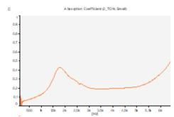
Fig.13. Absorption Coefficient of Composite of Carton-Zeolite as function frequency
