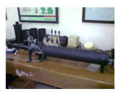
Fig. 11. impedance Tube type 4206 T
