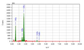
Fig. 17. EDS spectrum of Composite HVS-Zeolite
