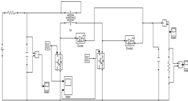
Fig. 8: Matlab/Simulink Model of Proposed Dc-Dc Converter in Open-Loop Method.
