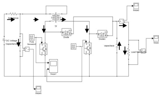
Fig. 2: Mode 1 Circuit Diagram.
