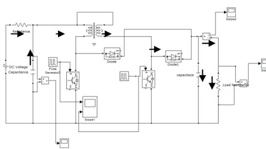
Fig. 3: Mode 2 Circuit Diagram.
