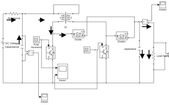
Fig. 5: Mode 4 Circuit Diagram.
