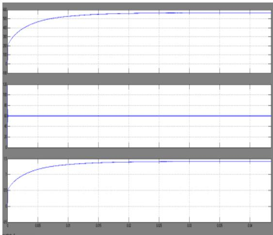
Fig. 9: Waveforms of Output Voltage, Input Voltage and Output Current of Dc-Dc Converter in Open-Loop Method.
