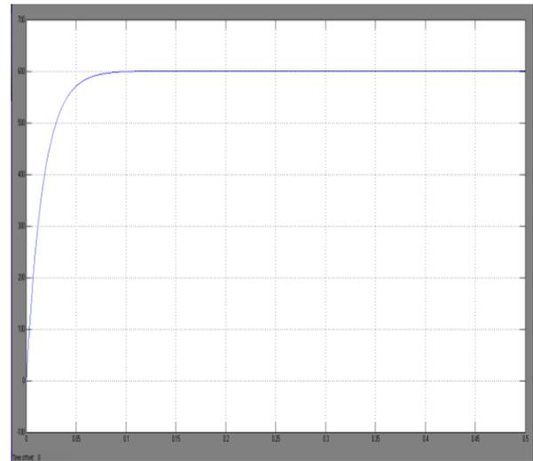
Fig. 11: Shows the Output Voltage of Proposed Dc-Dc Converter in Closed-Loop Method with Fuzzy Controller.
