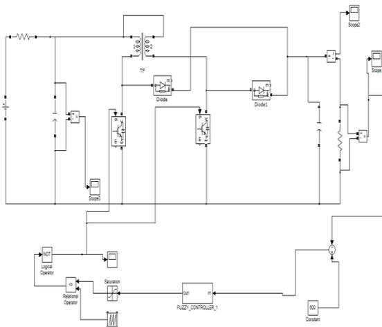
Fig. 10: Matlab/Simulink Model of Proposed Dc-Dc Converter in Closed-Loop Method with Fuzzy Logic Controller.
