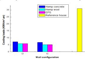
Fig. 19: Cooling Loads for the Least and the Most Efficient Configurations.
