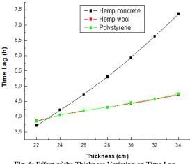
Fig. 6: Effect of the Thickness Variation on Time Lag.
