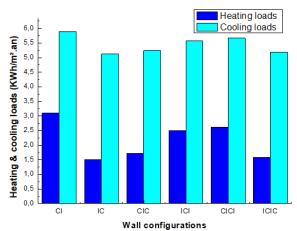
Fig. 16: Heating & Cooling Loads for an Insulated Building with Hemp Wool.
