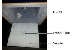
Fig.3: The Box B1 Used for Thermal Conductivity Measurement.
