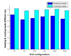
Fig. 15: Heating & Cooling Loads for an Insulated Building with Hemp Concrete.
