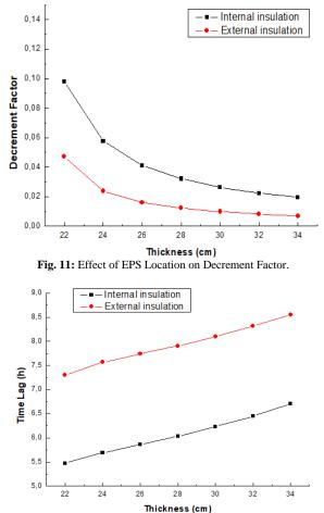
**Fig. 12:** Effect of EPS Location on Time Lag.
