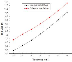
Fig. 8: Effect of Hemp Concrete Location on Time Lag.
