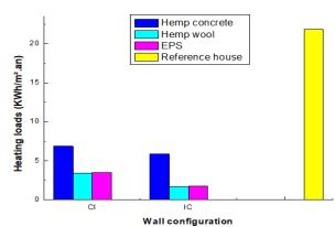
Fig. 18: Heating Loads for the Least and the Most Efficient Configurations.
