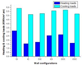
Fig. 17: Heating & Cooling Loads for an Insulated Building with EPS.
