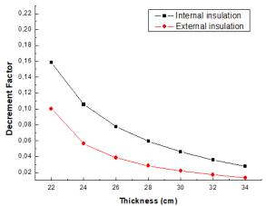
Fig. 7: Effect of Hemp Concrete Location on Decrement Factor.
