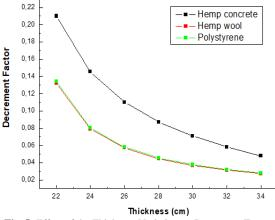
Fig. 5: Effect of the Thickness Variation on Decrement Factor.
