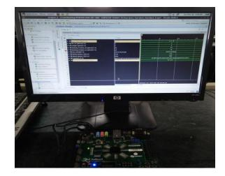
**Fig. 15:** Physical view of implementation Reconfigurable DNA Crypto System through Pseudo Biotic Key Encryption Mechanism on Zed Board (Zync Architecture).
