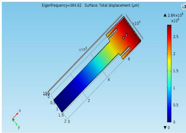
Fig. 4(a): Two Square perforations on cantilever at free end
