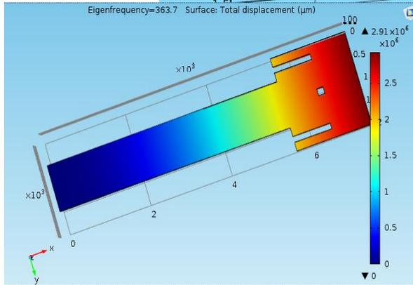
Fig. 3(a): Square perforations on cantilever at free end
