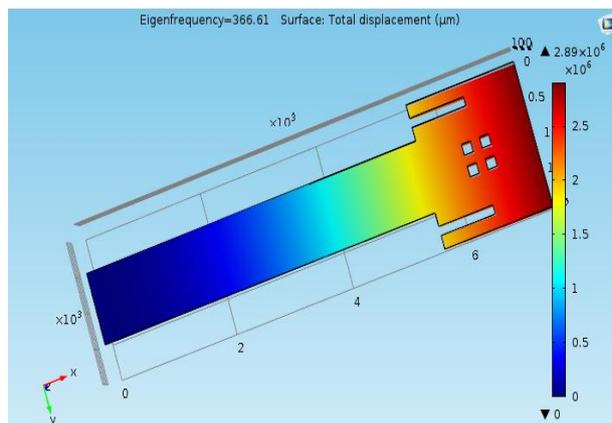
Fig.5(b): Four circular perforations on cantilever at free end
