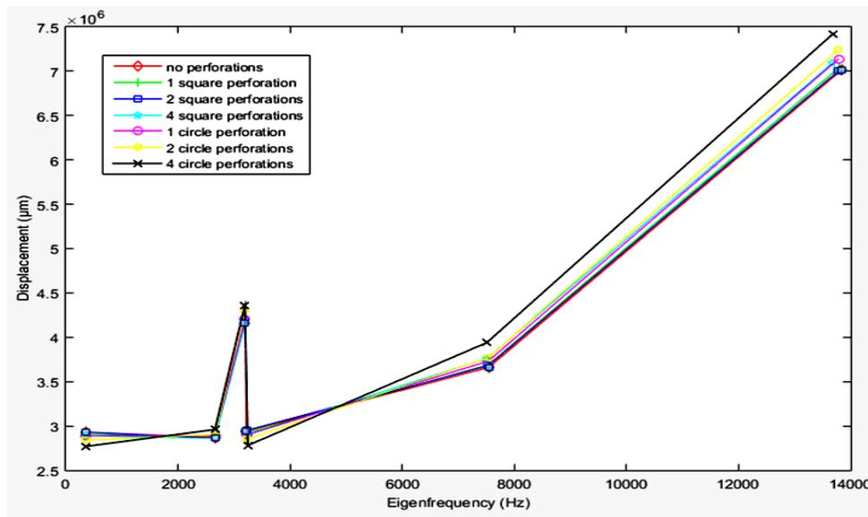
**Fig. 6:** variation of Displacement with variation in Eigen Frequency for different types of perforations.
