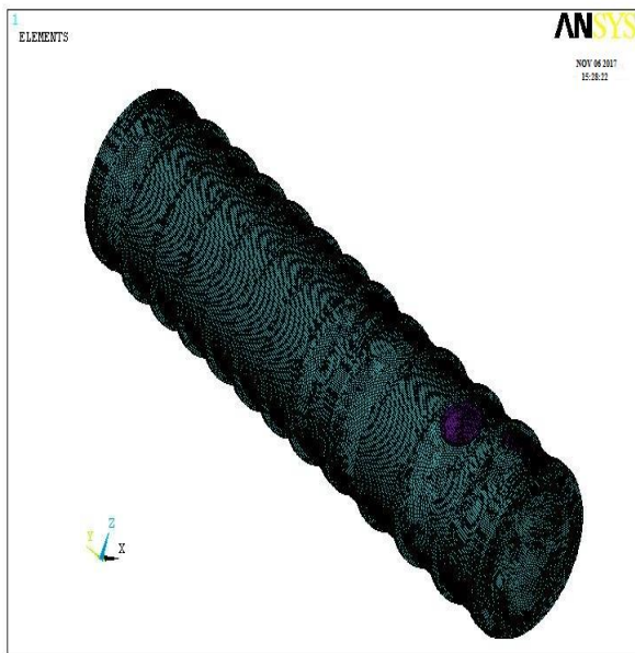
Fig.5: The above figure shows the complete constrained outside of the hull by using Shell 63 Element
