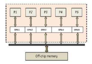
Fig. 5: Architectural model of five processors
