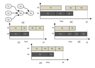
**Fig. 7:** (a) TDG. Schedule based on (b) no L2 cache, (c) equal partitioned L2 cache, (d) non-equal partitioned L2 cache, (e) integrated approach
