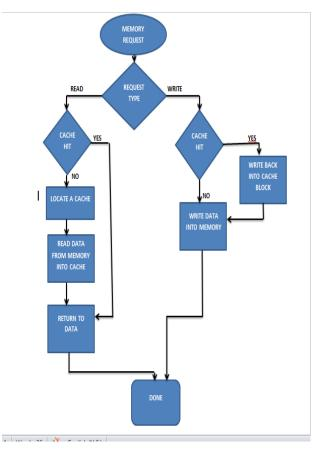
Fig. 10: Flow diagram of L2 Cache System
