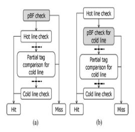
**Fig. 2:** Hot Hit Ratio Based Multistep Tag Comparisons (a) Medium/low Hot Hit Ratio. (b) High Hot Hit Ratio
