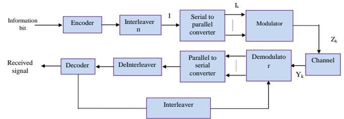
Figure 1: Block diagram of the BICM-ID system
