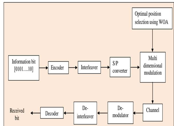
Figure 4: Overall diagram of proposed methodology
