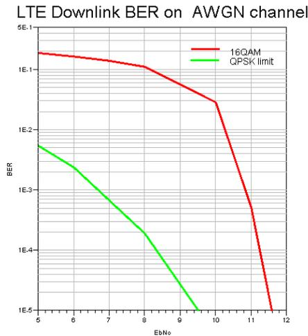
Fig 2: LTE Downlink Receiver BER on AWGN channel
