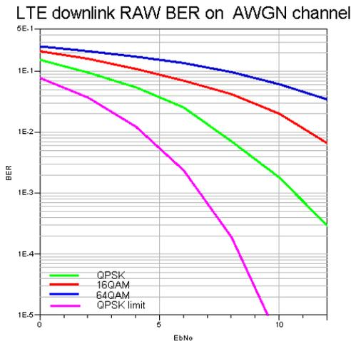
Fig 4: LTE Downlink Receiver Raw BER on AWGN channel
