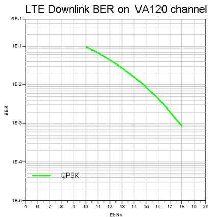
Fig 3: LTE Downlink Receiver BER on VehA channel
