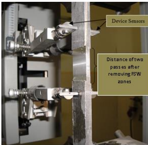
Fig. 1: Tensile specimen on tensile device after removing the FSW zones.
