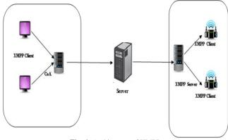
Fig. 4: Architecture of XMPP.
