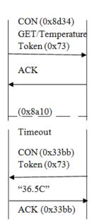
Fig. 9: GET Request with Separate Response.
