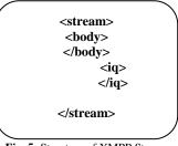
Fig. 5: Structure of XMPP Stanza.
