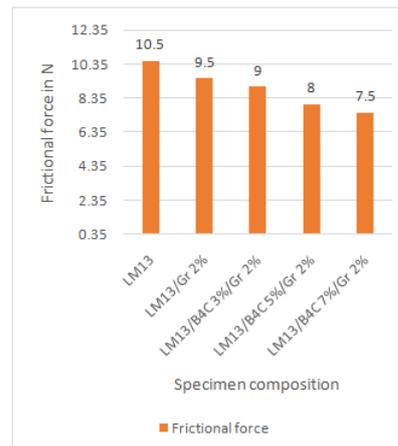
Fig. 16: Frictional force of pin on disc test specimens
