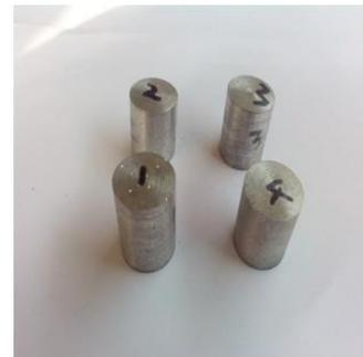
Fig. 8: Hardness test specimens
