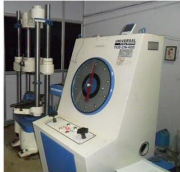
Fig. 5: Universal testing machine.
