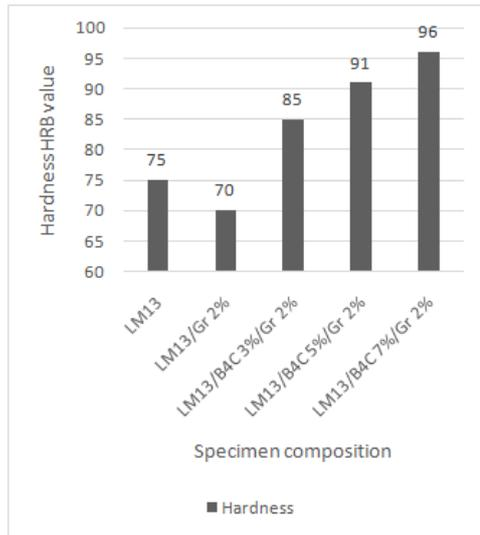
Fig. 13: HRB value of hardness test specimens
