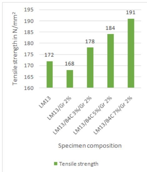
Fig. 11: Tensile strength of tensile test specimens
