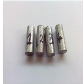
Fig. 10: Pin on disk test specimens
