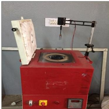
Fig. 1: Stir casting equipment
