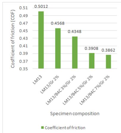
Fig. 15: COF value of pin on disc test specimens
