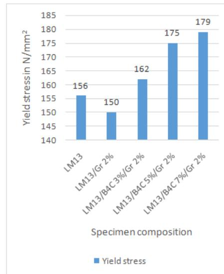
Fig. 12: Yield stress of tensile test specimens reinforcement results in increase in yield stress by 11% and 13% respectively.
