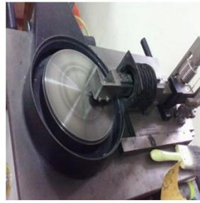
Fig. 9: Pin on disk testing machine
