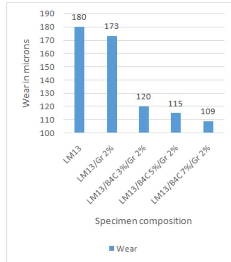
Fig. 14: Wear of pin on disc test specimens
