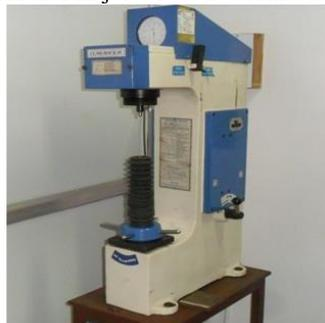
Fig. 7: Rockwell hardness testing machine
