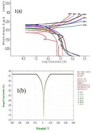
Fig. 1: Polarization Curves for (A) Ni-P Coatings (B) Ni-B Coatings.
