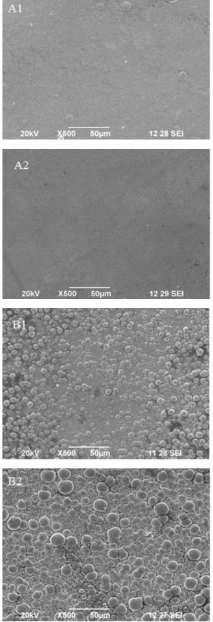
Fig. 5: SEM for Ni-P Coating ANNEALED at (A1) 300°C (A2) 500°C and Ni-B Coating Annealed at (B1) 300°C (B2) 500°C.
