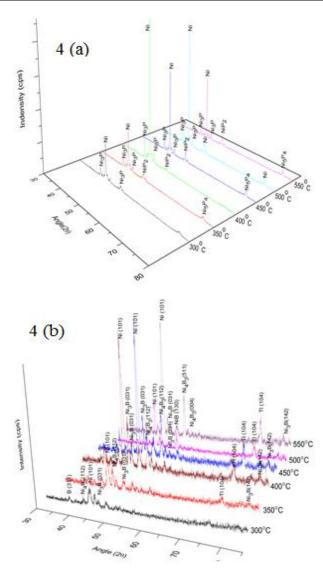
Fig. 4: XRD of Annealed Electroless Coatings (A) Ni-P (B) Ni-B.
