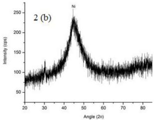
Fig. 2: XRD of As-Coated Electroless Coatings (A) Ni-P (B) Ni-B.
