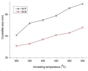
Fig. 6: Comparison of Crystallite Sizes of Ni-P and Ni-B Coatings.
