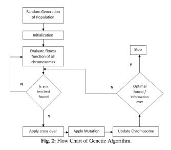
Fig 2 shows the genetic algorithm flow chart. Random generation of 50 chromosomes is done by random bit generator. The validation of the random bit are done at initialization process and the values are initialized by the random combination of the communication link. The design of the fitness function is done from the problem of the optimization which is given below. Optimization problem:
