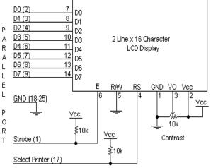
Fig. 5: Pin Diagram of LCD.
