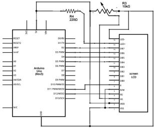
Fig. 6: LCD and Aurdino Interfacing.
