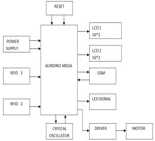
Fig. 2: Automatic Toll Gate Billing System's Block Diagram.
