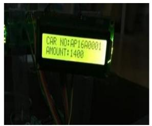
Fig. 9: Car Number and Account Balance Display.
