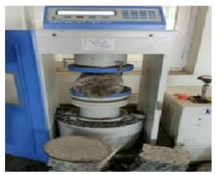
Fig. 4: Showing Cylinder Testing.
