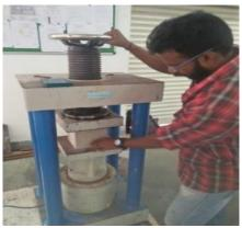
Fig. 5: Compression Test Machine.
