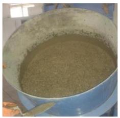
Fig. 2: Fresh Geopolymer Concrete.
