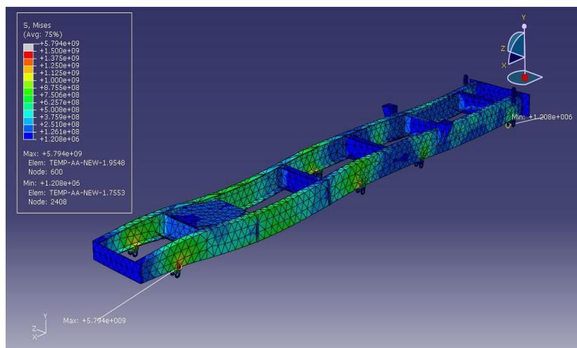
Fig. 2: Chassis after Loading, Analyzing and Displaying Critical Tensions.
