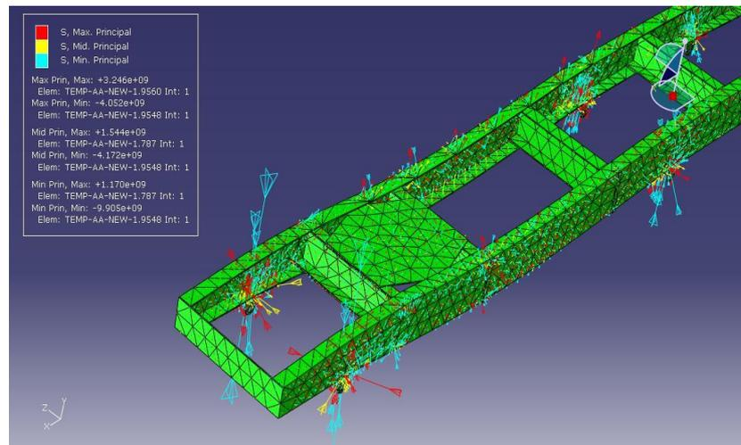
Fig. 3: Distribution the Stress Tensor on the Chassis in A Static State.
