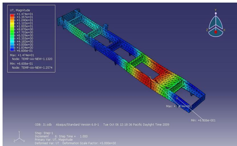
Fig. 4: Displacement Values of Chassis Points after Loading.
