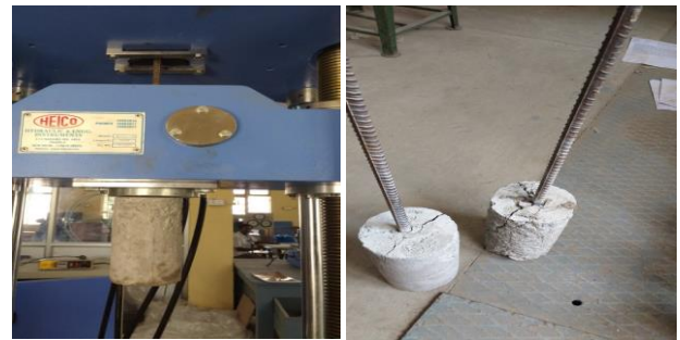
Fig. 2: Snapshot for Pull out Test Specimens.
