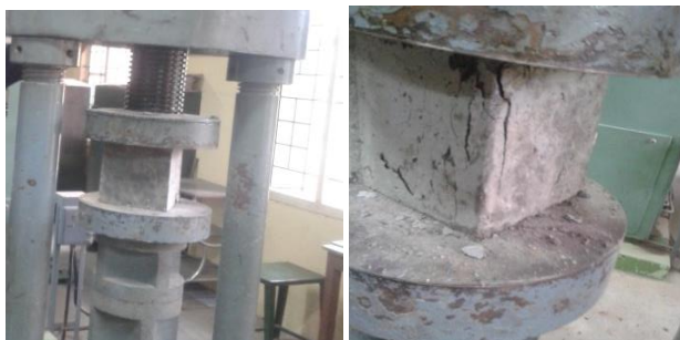
Fig. 1: Snapshot for Testing of Compressive Strength of Concrete.
