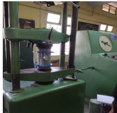
Fig. 3: Snapshot for Modulus of Elasticity of Concrete.
